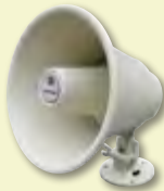
AH-108 Horn Speaker • 8Ω, 10W • Indoor or outdoor use • Surface mount Bell Diameter: 6-1/8" Depth: 6-1/2"
