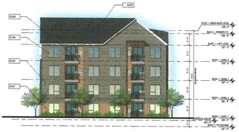
11 BUILDING 1 - OVERALL BUILDING ELEVATION - WEST Scale: 1/8" = 1'-0"
