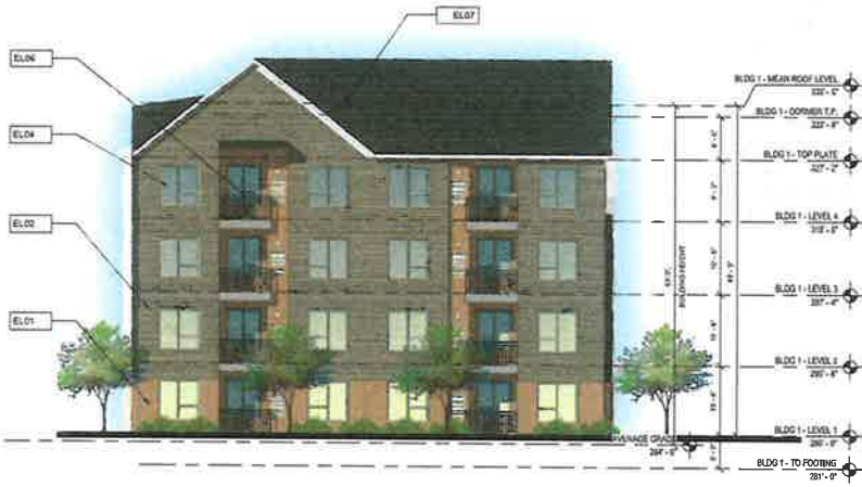
11 BUILDING 1 - OVERALL BUILDING ELEVATION - EAST Scale: 1/8" = 1'-0"
