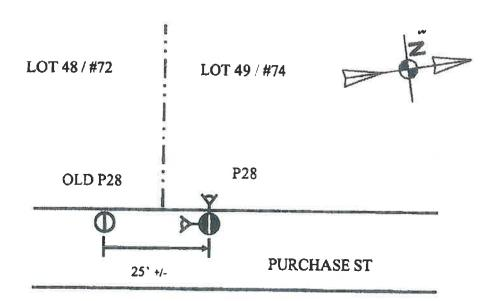
NATIONAL GRID RESPECTFULLY REQUEST PERMISSION TO REPLACE AND RELOCATE POLE 28 (25') NW OF PRESENT LOCATION IN ORDER TO REMOVE TREE GUY FROM #74 PURCHASE ST. OLD LOCATION DOES NOT WORK DUE TO CUSTOMERS RETAINING WALL.
